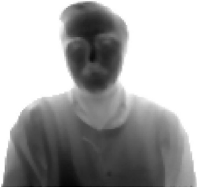
Figure 2. Distance image of a face. We notice that the moustache and the eyebrows are whiter, hence farther than the rest of the face.
